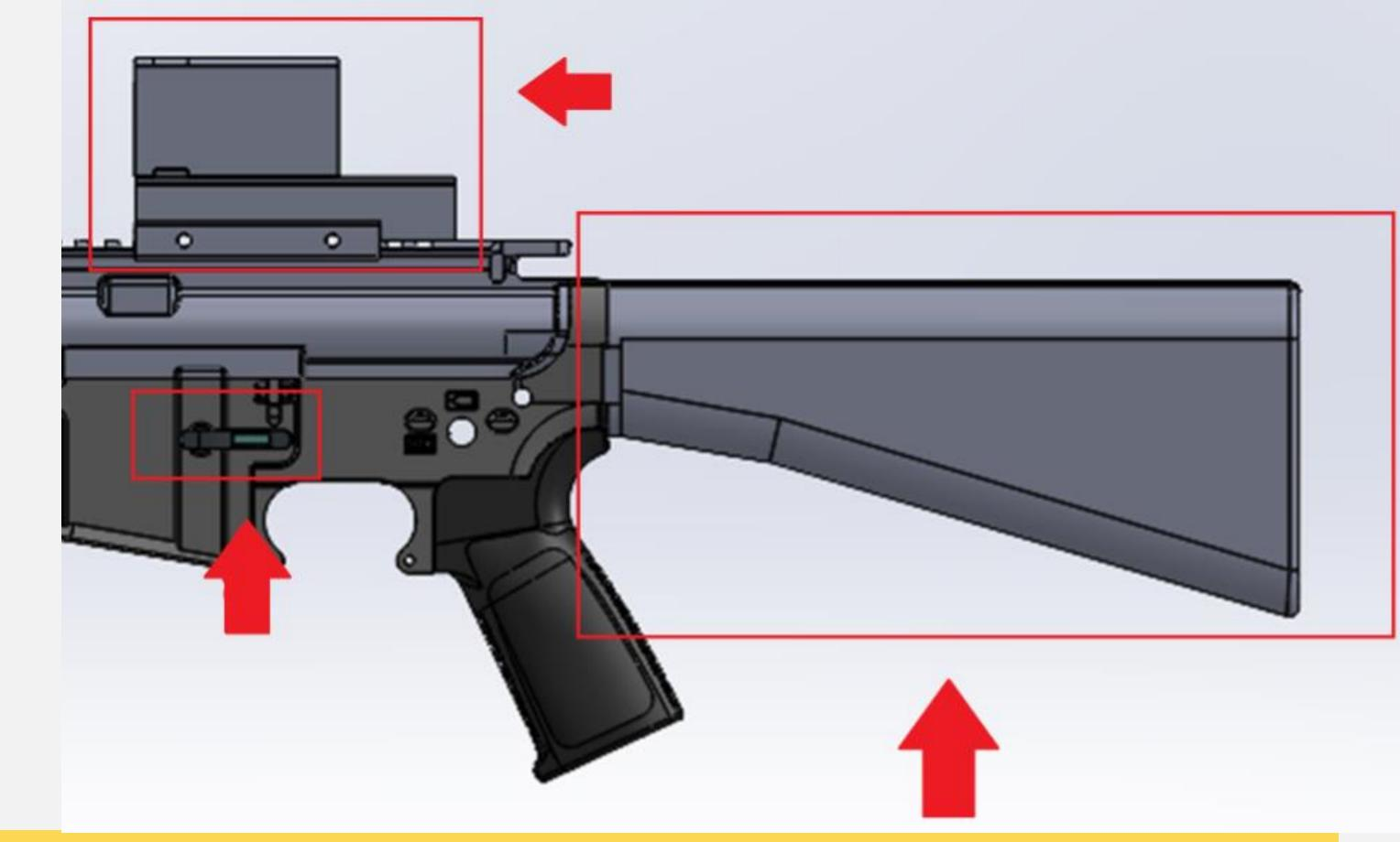
Cerberus replaces the stock, magazine release, and optic on the AR platform, tracking rounds fired to help operators maintain their rifle and stay aware of their ammo during critical operations.
